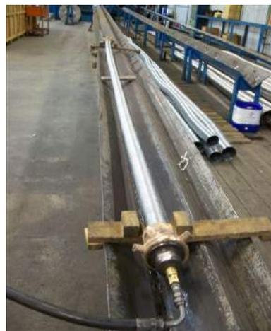
Stripwound bitumen hose being pressure tested
