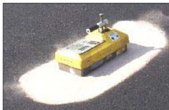
Figure 1: Nuclear Density Testing
