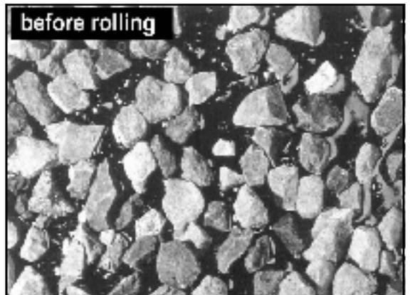
Figure 1. Correctly spread aggregate before rolling
