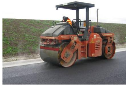
*Tandem, steel-wheeled vibratory roller.*
